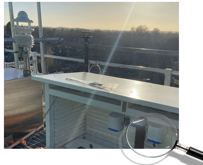
Fig. 1: The temperature sensor is integrated in the PM module of the AirGradient monitor. To test the impact of the sensor position, an additional sensor was added outside of the monitor box. Both sensors were compared to a reference device.
