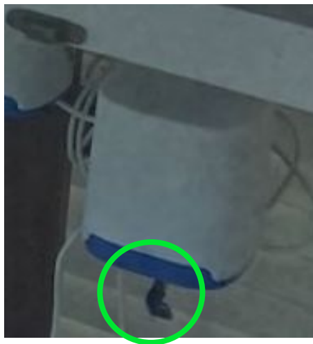
Fig. 1: The temperature sensor is integrated in the PM module of the AirGradient monitor. To test the impact of the sensor position, an additional sensor was added outside of the monitor box. Both sensors were compared to a reference device.
